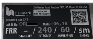
It is important to be specific when ordering a fire door. Always specify the full fire resistance rating, for example -/120/60 minutes FRR. We have seen cases where the door may have been specified as a “two-hour fire rated door”, and indeed one has been installed, but unfortunately is -/120/30, or -/120/- which, while having a two-hour element, are not sufficiently rated for the regulations (they are deficient in the insulating property).
